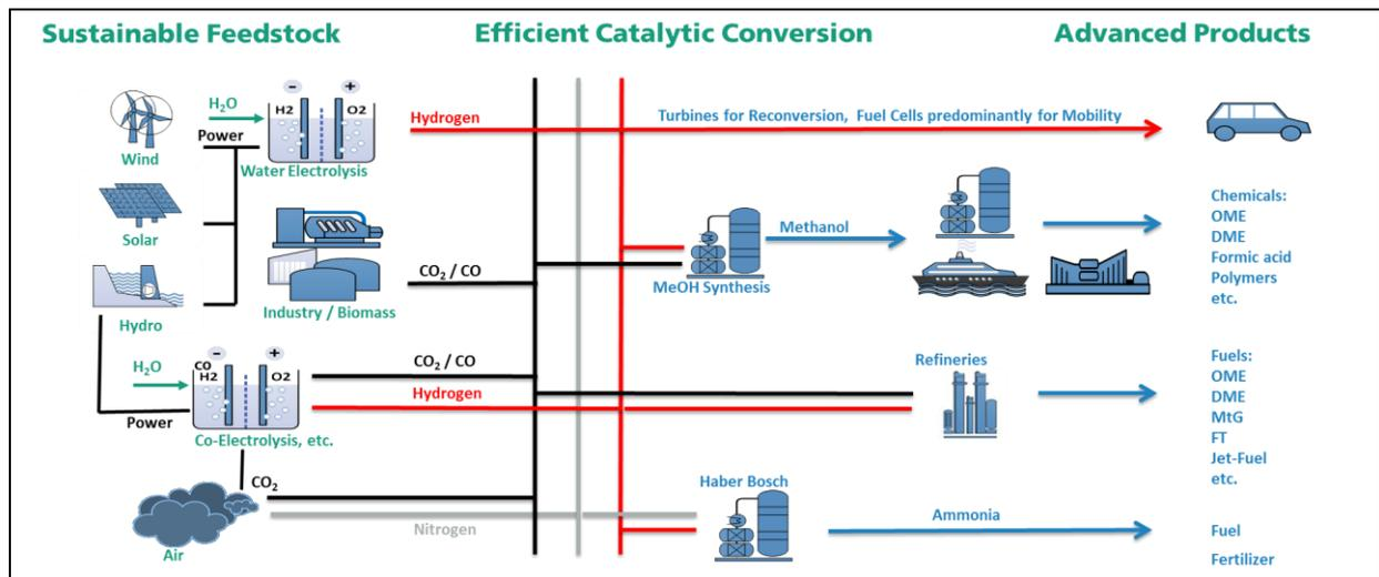
Fig 1: Power-to-X process chains
