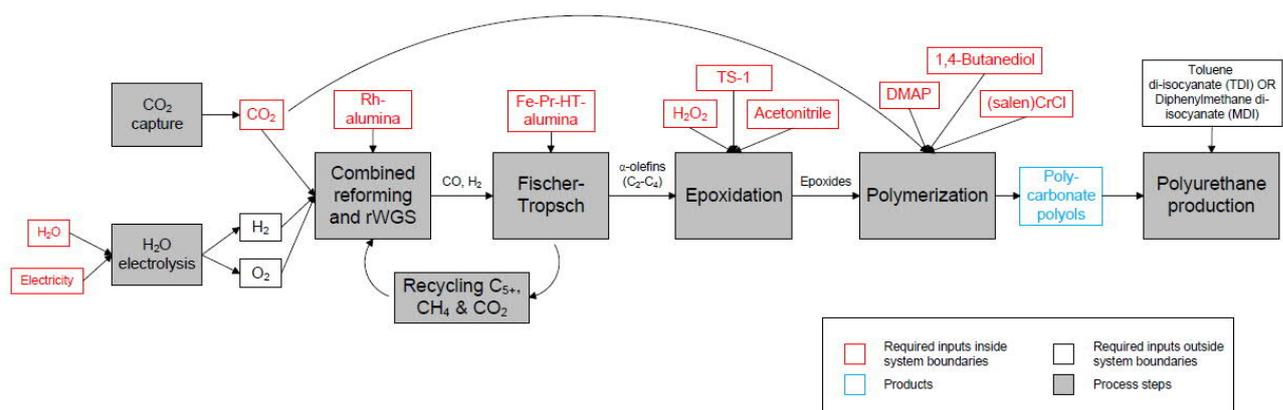
**Figure 1. A simple flowchart of the BECCU process.**
